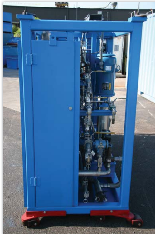
Side view of RWRO™ skid with integrated shielding and hinged shield doors for easy access to housings for membrane changeout.
