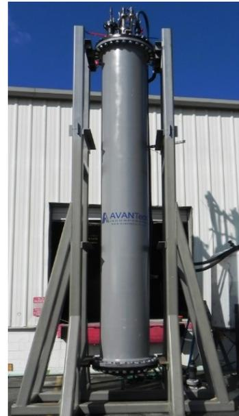
CST was a specialty resin developed in the 90s by DOE Sandia National Laboratories and Texas A&M University. It was later licensed by DOE for commercialization to Honeywell UOP. CST exchange media is a single-use material that cannot be regenerated, but it is very selective for the cesium isotope in a salt environment and has an extremely high loading capacity. Once fully loaded with cesium-137, the spent CST resin is removed and the vessel is replaced or replenished with fresh resin.
