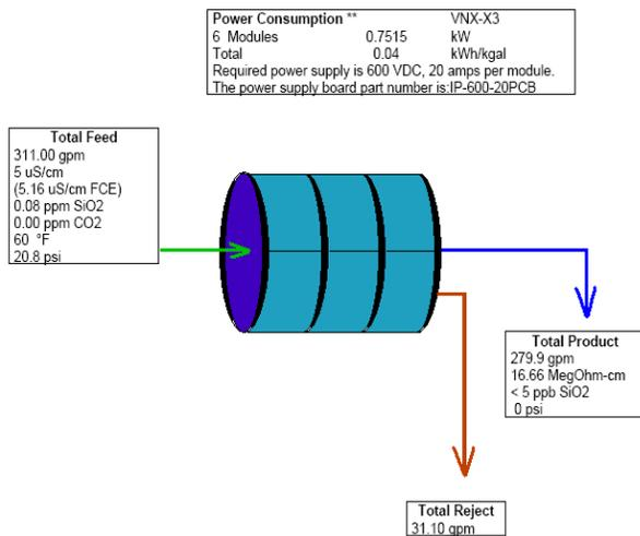
The EDI system will produce a permeate flow of 280 gpm. The system requires a feed rate of 311 gpm combined with a 10% reject flow of 31 gpm. The EDI permeate will pass down stream to the client supplied storage tank at 60 psig.
