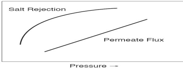
Operation of a membrane system at higher fluxes results in lower permeate salt concentrations and a better permeate quality. At the lower recycle permeate flow of 243 gpm, the average membrane flux is 9.7 gfd, which is approximately 22% lower than the design flux of 12.4 gfd. This lower flux allows the ratio of salts to water in the permeate to increase, thus lowering the RO permeate quality.
