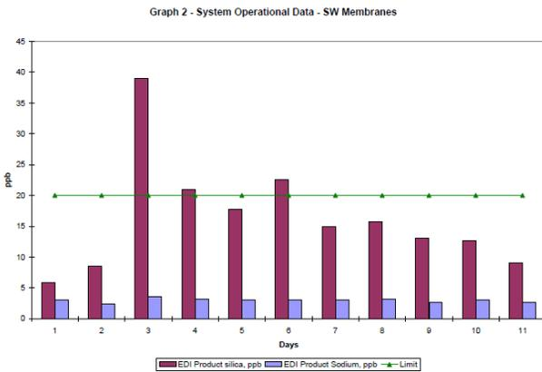
The CO<sub>2</sub> & SiO<sub>2</sub> on the RO permeate in ppm, SiO<sub>2</sub> and Na on the EDI permeate are display in ppb.
