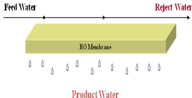
The principle of RO is based on the solution - diffusion model, which states that water transport is a function of the net driving pressure and membrane water permeability, salt transport is function of the concentration differential and the membrane salt permeability. Salt flux divided by water flux equates to the permeate concentration. Relatively speaking, this means that salt transport is not pressure or flux dependent, but water transport is highly pressure/flux dependent.
