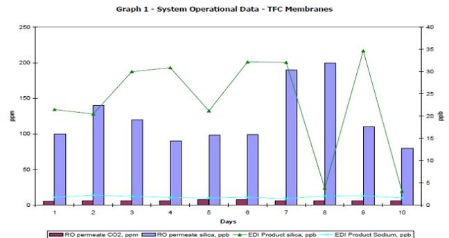
The CO<sub>2</sub> & SiO<sub>2</sub> on the RO permeate in ppm, SiO<sub>2</sub> and Na on the EDI permeate are display in ppb.
