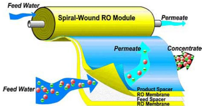
ROS membranes are hydraulically designed for cross-flow versus a cartridge filter, which would be straight-through or dead-end filtration. The pressurized feed stream enters the RO membrane and flows parallel to the membrane surface as shown in the following illustration.
