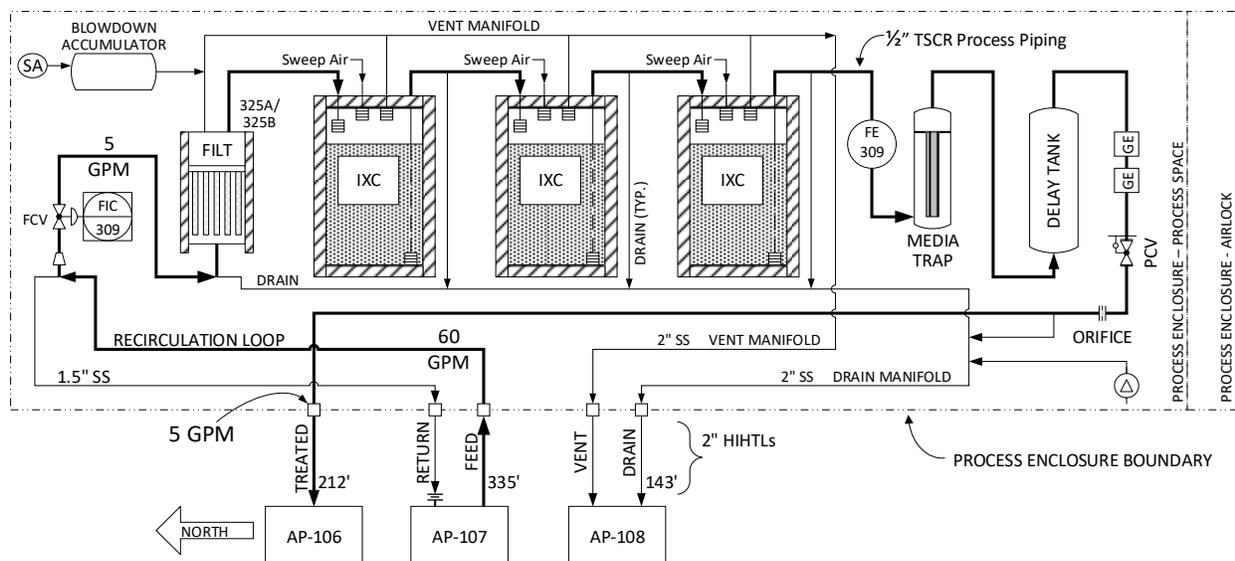
Fig. 5. TSCR Flow Diagram.
