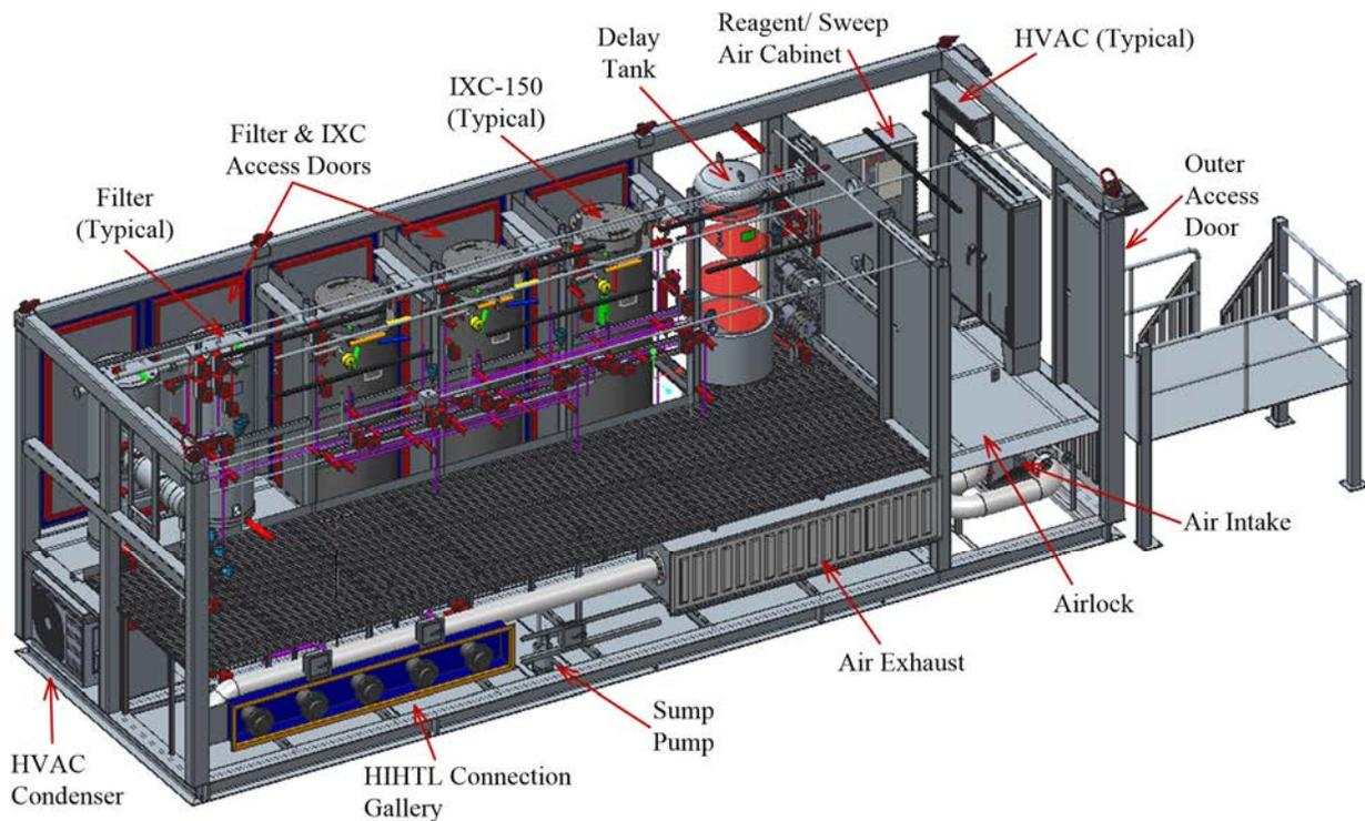
Fig. 6. Process Enclosure Arrangement.
