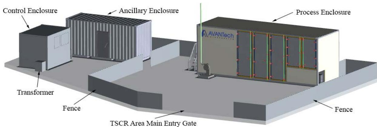
Fig. 4. TSCR System General Arrangement.
