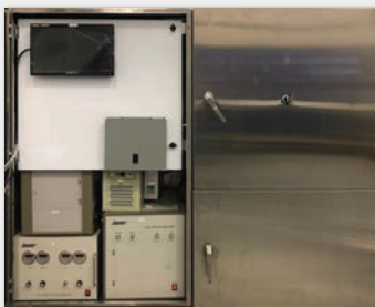
Continuous Emissions Monitor (CEM) Smart Sampler System
